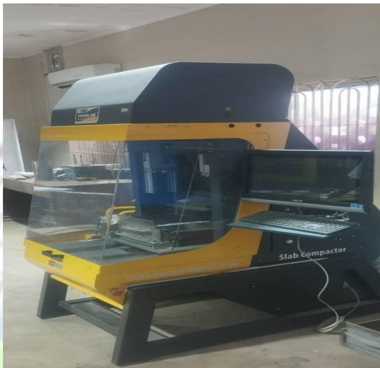
Slab Compactor: Used to measure asphalt slab specimen
