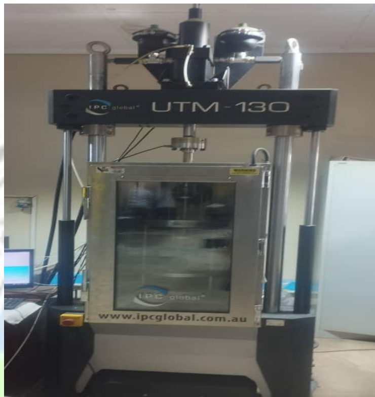
Universal Testing Machine for testing Soil and Asphalt (Stress and Strain behavior)
