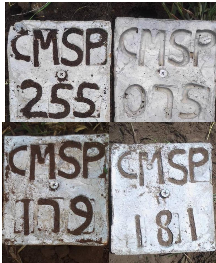
<Figure 3-8: Installed Secondary survey control markers between Chalinze and Morogoro>
